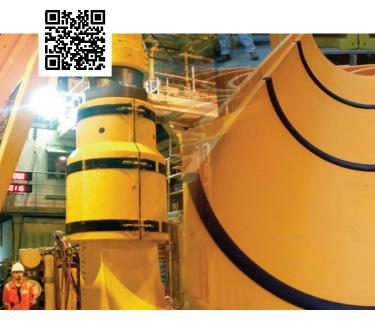
Unlike linepipe or cast-in-place insulation which is designed for hot-dry service, half-shell shrouds, housing, clamp and retro-fit insulation products ensure hot-wet service as the cavity between the structure and insulation is flooded with seawater. Balmoral Elastotherm® can provide suitable hot-wet performance over a design life of up to 30 years.
